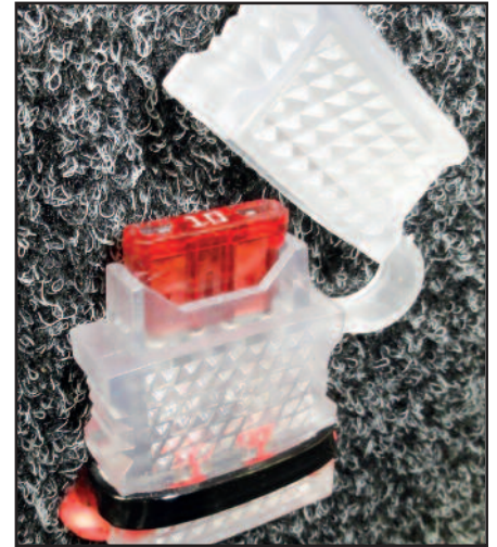
TX fuse (in cab) and the Vito fuse (on carpet) should be disconnected before a jump start
